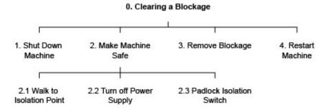
The next step is to draw up "plans" which specify the order in which the operations should be carried out. Plan 0, for example, would be "Do steps 2 to 4, if blockage cleared, continue, if blockage remains repeat steps 1 to 4 in order". Plan 2 would be "Do steps 2.1 to 2.3 in order".
