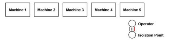
Redesigning the controls increases the likelihood that the operator will follow the safe working procedure and isolate the machine before clearing a blockage.
